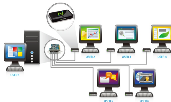
One X550 Kit Enables Six Users to Share a PC (Eleven with Two Kits)
