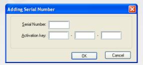
Enter the serial number and the activation key of the first terminal. Click on the "OK" button. Click on the "Add" button again to add another terminal's information, and so on. It is recommended to enter information for each terminal connected to the host PC at this time. They can be added later.
